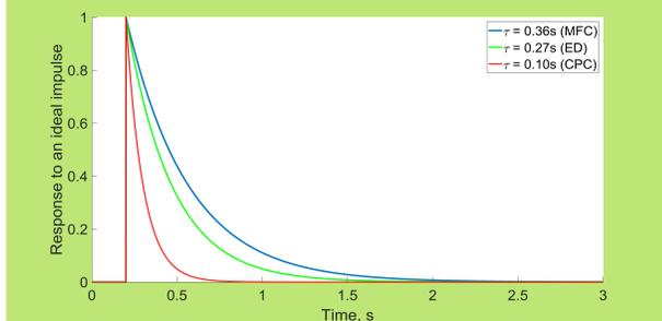
→The combined effect is a rapid increase in the sample flow, followed by settling to a level determined by the ejector diluter pressure dependence.
